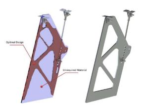
One example of GRM's capabilities in the MotorSport sector, is a recent development of the rear wing stay for a RoadSports prepared BMW Z3 race car. This short term project, delivered in only 2 days, demonstrates GRM's ability to apply their optimisation software tools to deliver minimum weight and practical designs. In this particular project TruForm SW was used to guide the development of a design able to support aerodynamic and abuse loading. The completed
